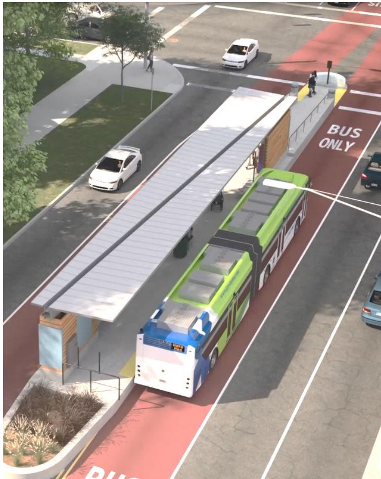
Figure 8-7. BRT Station Concept – Curbside BAT Lanes
